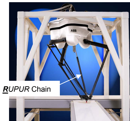
Figure 1. ABB Robotics FlexPicker with its remote actuation.
