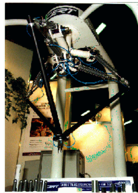
Figure 4. Speed-R-Man, a kinematically redundant PKM.
