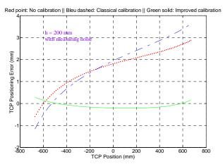
Fig. 6 – TCP positioning before and after classical and improved calibration
