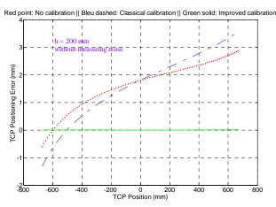
Fig. 7 - TCP positioning before and after classical and improved calibration.
