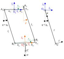
Fig. 3 – Scheme of the simple mechanism. Left: exact mechanism. Right: equivalent simplified mechanism used for the computation of the models
