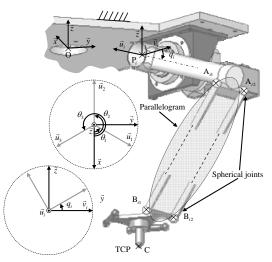
Fig. 1 - Scheme of a pair of rods of the Delta robot
