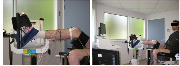
Fig. 2. Electrodes configuration (left) and experimental set-up (right).
