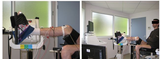
Fig. 1. Experimental set-up for electrical stimulation and ankle torque measurement.
