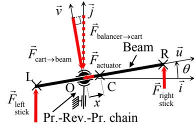
Fig. 6. Scheme of the force sharing device: the force produced by the balancer is shared between the right and the left sticks depending on  $x$ . Pr. and Rev. stand for Prismatic and Revolute joints, respectively.
