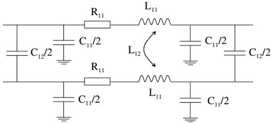
Fig. 5: Elementary cell for coupled-line  $\pi$ -model.
