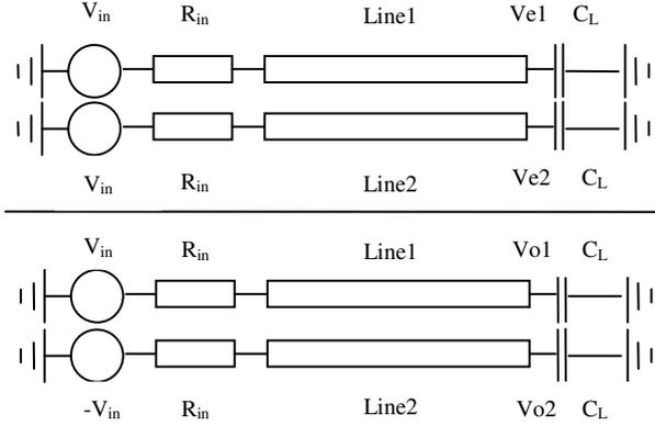
Fig.2: Coupled-line configurations for even and odd modes.
