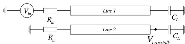
Fig. 1: Coupled-line model.
