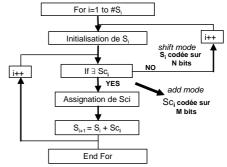
Figure 4: Algorithme de Compression
