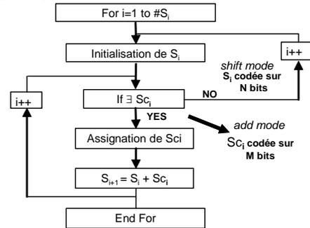
Figure 4: Algorithme de Compression
