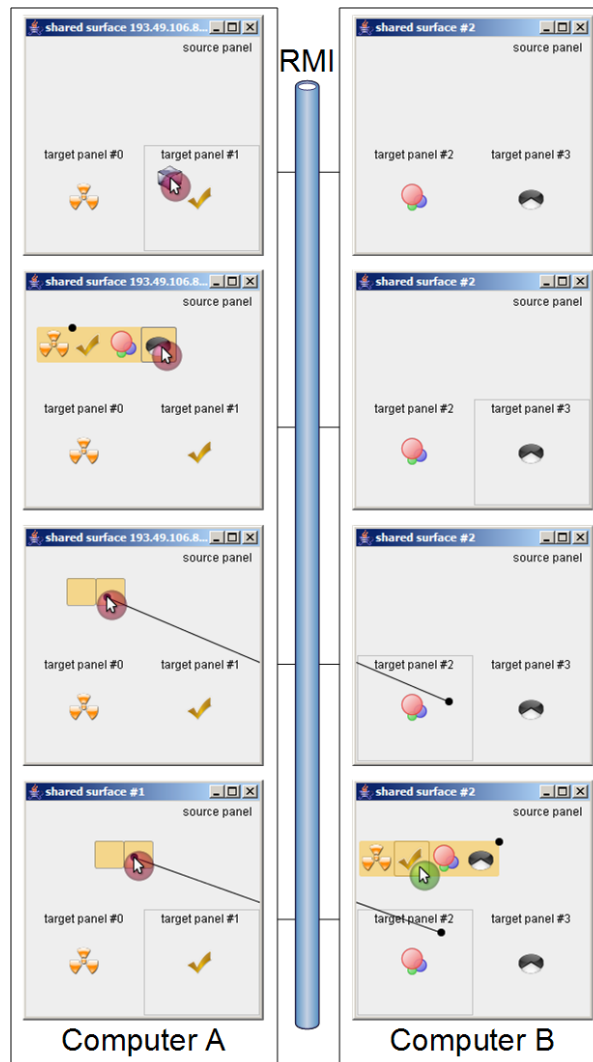
Fig. 5. (Top to bottom) (a) drag-and-drop (b) push-and-pop (c) push-and-throw (d) two concurrent manipulations: a push-and-throw from A to B and a push-and-pop from B to A.
