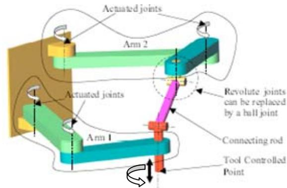
**Figure 15. The functioning principle of Dual4.**
