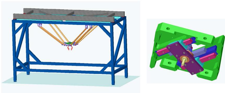
**Figure 11. I4L: a prototype with T-to-R transformation and a 3-part travelling plate**
