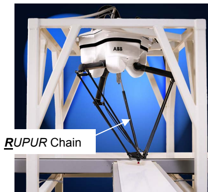
Figure 1. ABB Robotics FlexPicker with its remote actuation.
