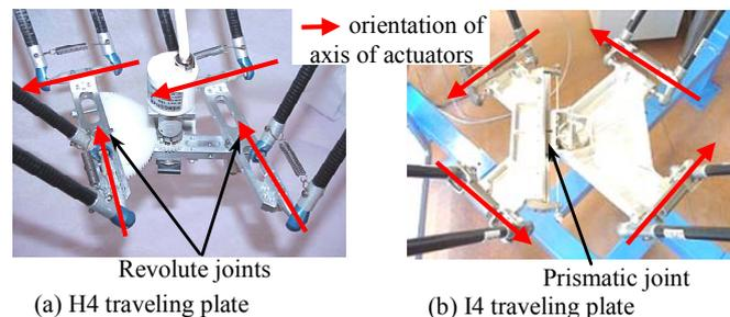
**Figure 9. Relative positions of  $(SS)_2$  chains for H4 and I4 mechanisms.**
