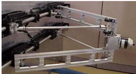
Figure 5. Archi: a 3-dof, 4-motors, actuation-redundant PKM.
