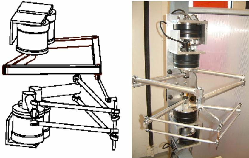
**Figure 16. One possible practical design of Dual4**
