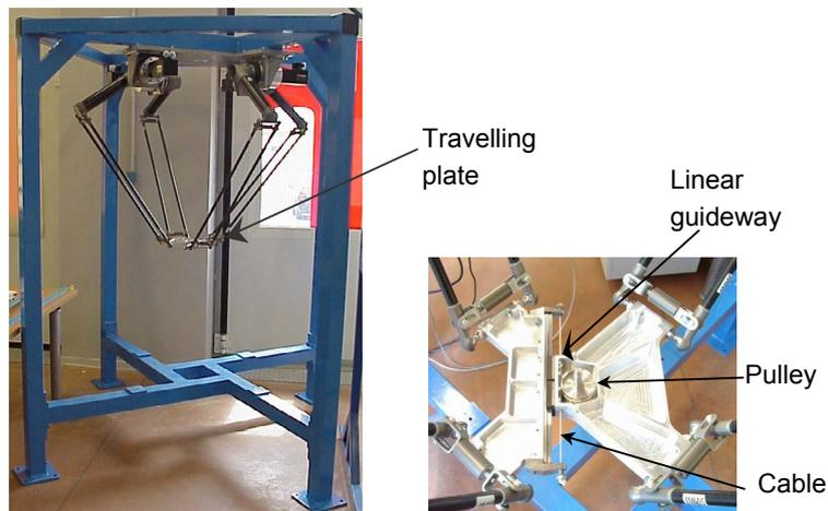
**Figure 10. I4R prototype (left) and its travelling plate with a prismatic passive joint (right).**
