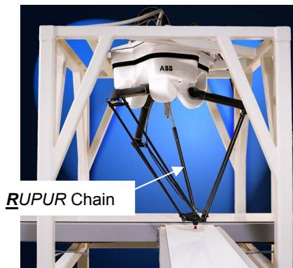
**Figure 1.** ABB Robotics FlexPicker with its remote actuation.
