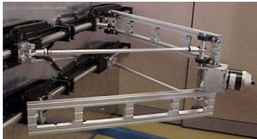
**Figure 5.** Archi: a 3-dof, 4-motors, actuation-redundant PKM.
