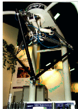
Figure 4. Speed-R-Man, a kinematically redundant PKM.
