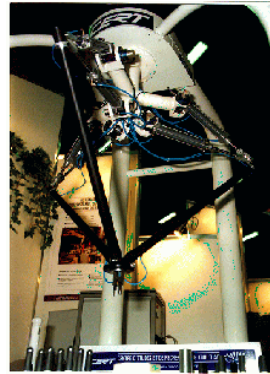
Figure 4. Speed-R-Man, a kinematically redundant PKM.
