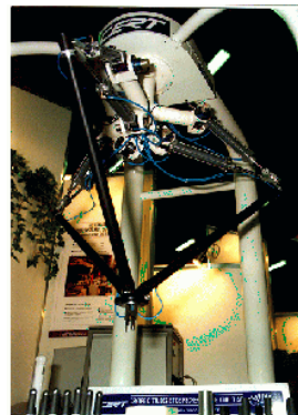
Figure 4. Speed-R-Man, a kinematically redundant PKM.
