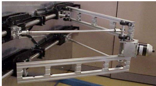
Figure 5. Archi: a 3-dof, 4-motors, actuation-redundant PKM.
