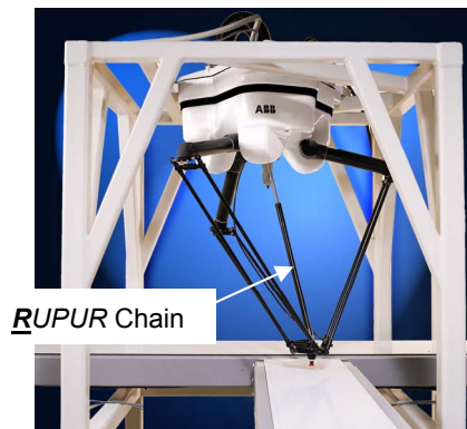
Figure 1. ABB Robotics FlexPicker with its remote actuation.
