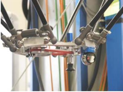
Fig. 3. Corner cube on the traveling plate
