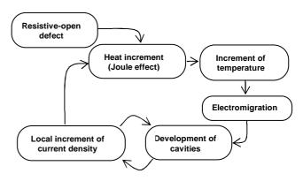
Figure 7: The acceleration electromigration cycle
