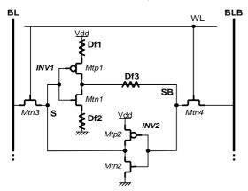
Figure 1: Resistive-open defects injected into the memory core-cell as cause of DRFs.
