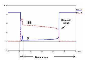
Figure 2: Data retention fault caused by high resistive defect Df1
