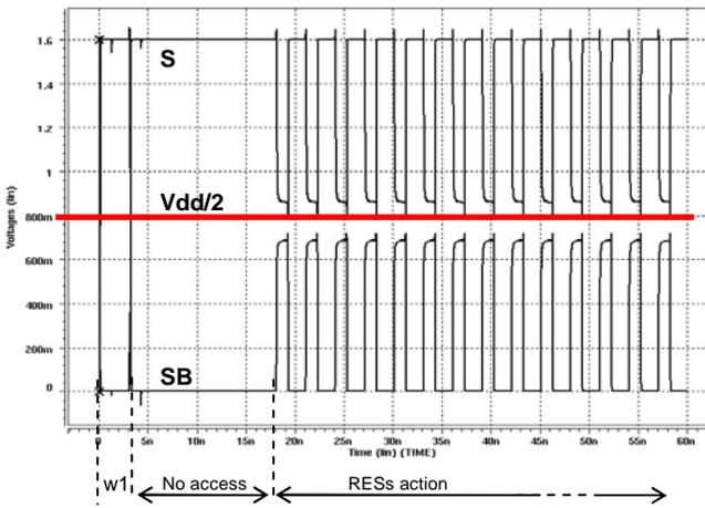
**Figure 6: Cell instability that may produce data retention faults. Df3 = 11.7kΩ**
