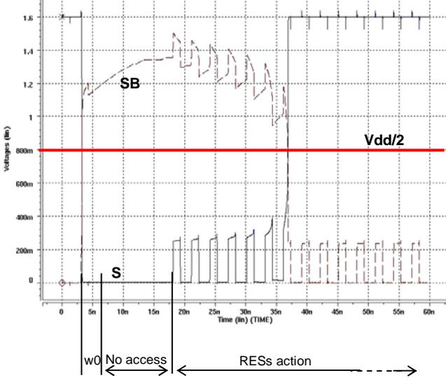
Figure 4: DRF caused by low resistive Df1
