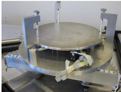
Fig. 8 Complete micro-stage with support in three points
