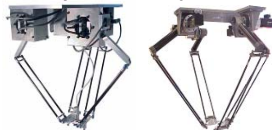
(a) H4 robot (b) I4R robot Fig. 1 Existing 4- dof prototypes
