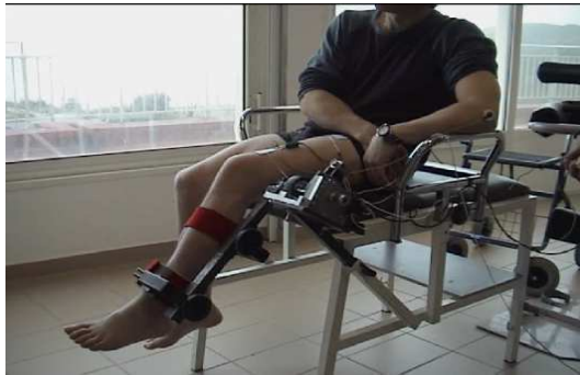
Fig. 10. Experiments on paraplegic patient during knee angle and torque measurements were performed at the Centre Bouffard-Vercelli (Cerbere - France)
