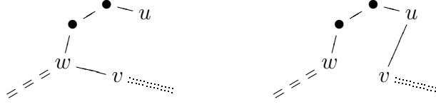
Figure 1: Turning the leaf u into a vertex of degree 2
