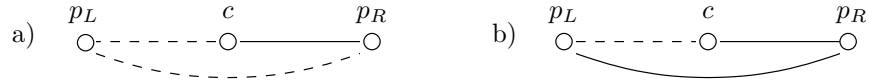
Fig. 8. In case a), the new center is p_R , in case b) p_L is chosen.
