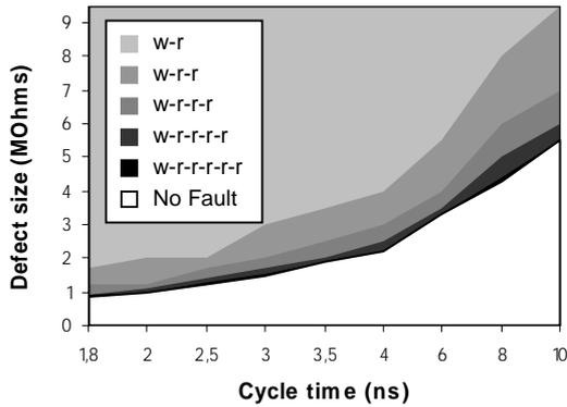
Figure 3: Fault detection as a function of the cycle time and defect size (typical process, T=125°C, V=1.6V)
