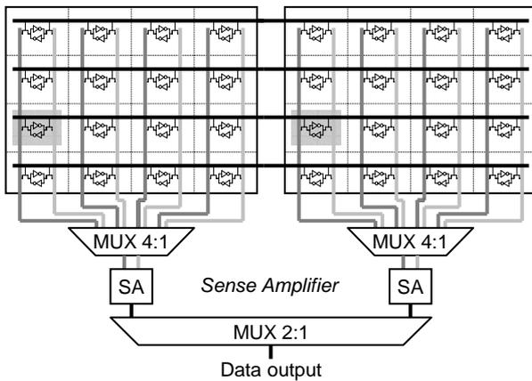
Figure 5: Scheme of a two-block SRAM memory
