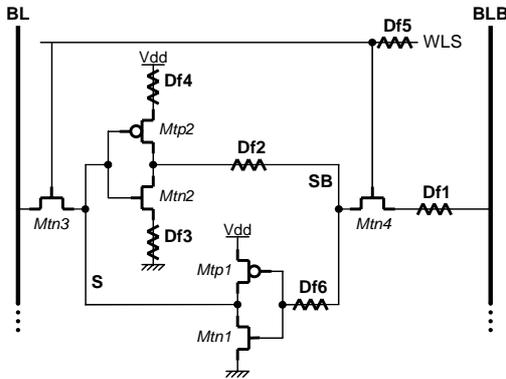
Figure 1: Resistive-open defects injected into the memory core-cell
