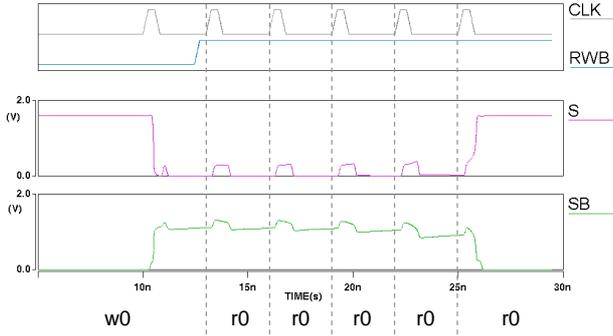
Figure 2: A destructive read occurring after the 5<sup>th</sup> consecutive r0 operation (typical process, T=125°C, V=1.6V, T<sub>cyc</sub>=3ns, R=1.5MΩ)
