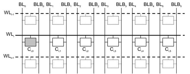
Figure 4: A portion of an SRAM block
