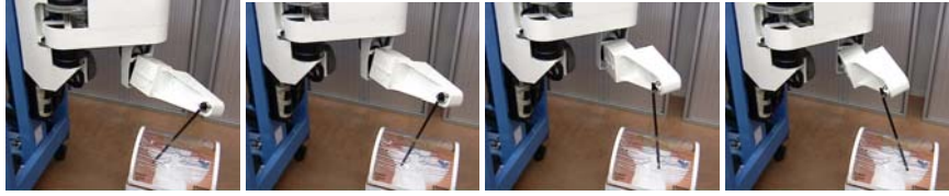
Fig. 6. Straight line motion of D2M2 under constraint of trocar
