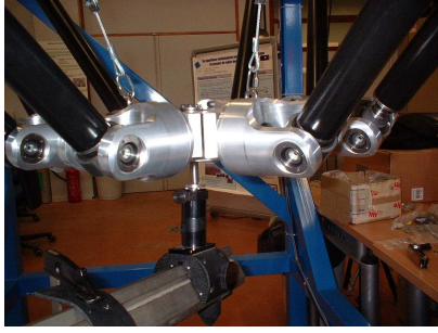
Figure 6: Experimental set-up for the straightness evaluation.
