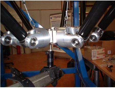
Fig. 9. Experimental set-up for the straightness evaluation.
