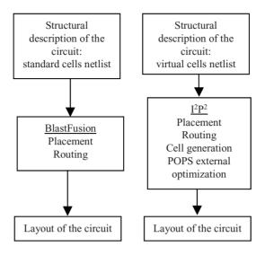
Fig. 4. Standard flow versus I<sup>2</sup>P<sup>2</sup>/POPS flow.
