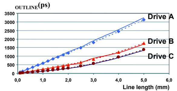
Fig.5. Simulated (full line) and calculated (dashed line) values of the line output transition time for the configuration specified in Table I, with different size of input drivers ( $R_{LINE}=115 \Omega/\text{mm}$ ,  $C_{LINE}=472 \text{ fF}/\text{mm}$ ).
