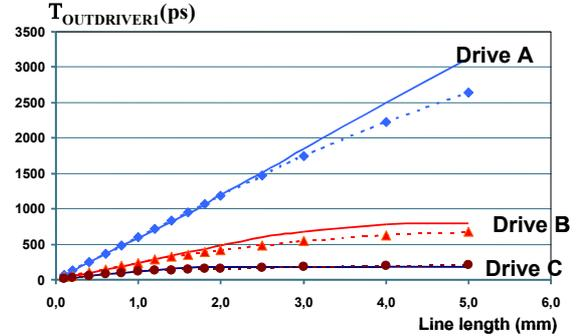
Fig.4. Simulated (full line) and calculated (dashed line) values of the input driver transition time for the configuration specified in Table I, with different size of input drivers ( $R_{LINE}=115 \Omega/\text{mm}$ ,  $C_{LINE}=472 \text{ fF}/\text{mm}$ ).
