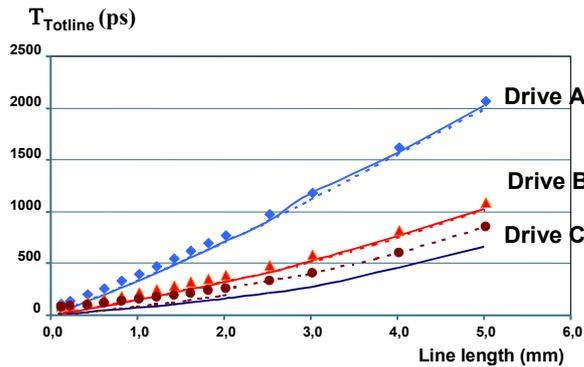
Fig.6. Simulated (full line) and calculated (dashed line) values of the total line propagation delay for the configuration specified in Table I, with different size of input drivers ( $R_{LINE}=115 \Omega/mm$ ,  $C_{LINE}=472fF/mm$ ).
