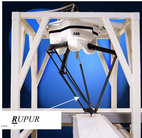
Figure 1. ABB Robotics FlexPicker with its remote actuation.
