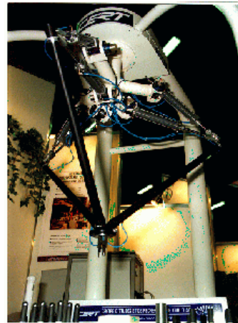
Figure 4. Speed-R-Man, a kinematically redundant PKM.
