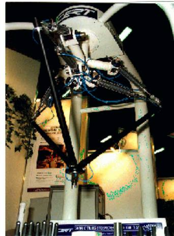
Figure 4. Speed-R-Man, a kinematically redundant PKM.
