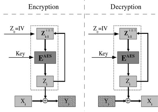
Figure 2: Encryption and decryption in OFB mode.
