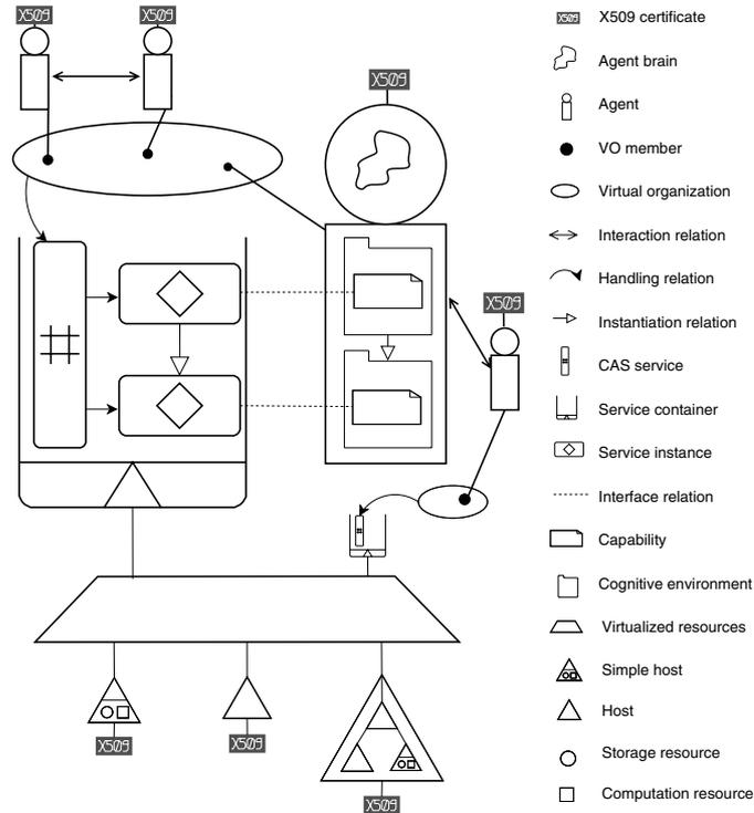
Fig. 1. The GRID-MAS integrated model described in AGIL’s graphical description language
