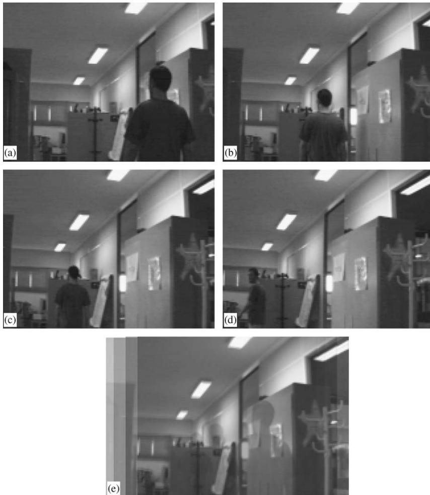
Fig. 20. Four images of the inside laboratory sequence (top and middle) with a character moving in front of the camera and their superposition according to the motion estimation (bottom).
