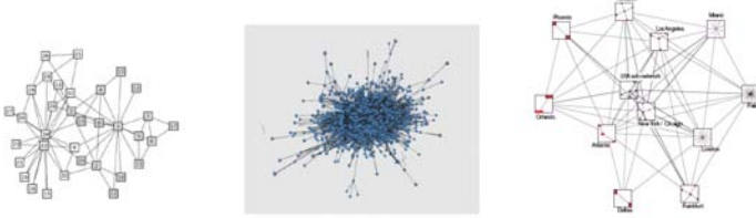
Fig. 2. Example layouts of force-directed algorithm on a small graph (left) and a larger graph (middle). The graph on the right has been clustered and then laid out using a force-directed method. (See also Fig. 4, Fig. 6 and Fig. 14.)
