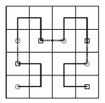
To end, all the starting and ending points are removed, except the starting point of the first copy and the ending point of the fourth copy.
