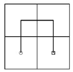
• From step n to step n + 1 the curve and grid sizes are decreased by a factor two and four copies are put together to form a new square.
