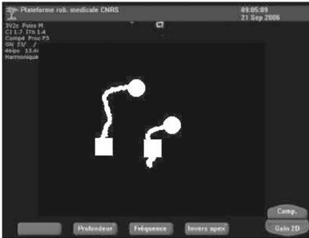
Fig. 19. Image trajectory for a complex motion between initial (circle) and desired (square) positions.
