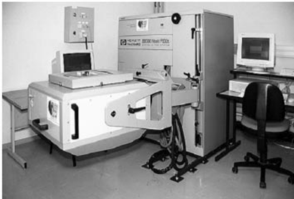
Fig. 2. Agilent 83000 F330t tester: test head (left), mainframe (centre) and workstation (right).
