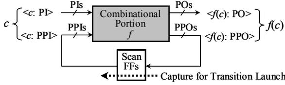
Fig. 14 Circuit Model for Launch-Induced Switching Activity.
