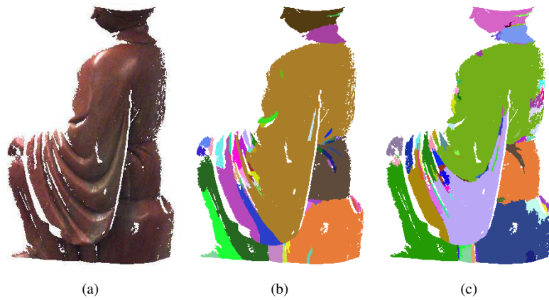
Fig. 5. Influence of the attribute space choice on the segmentation. Original range image (a). Segmented image in (b) angle between normal vector space, and (c) sphere fitting space.
