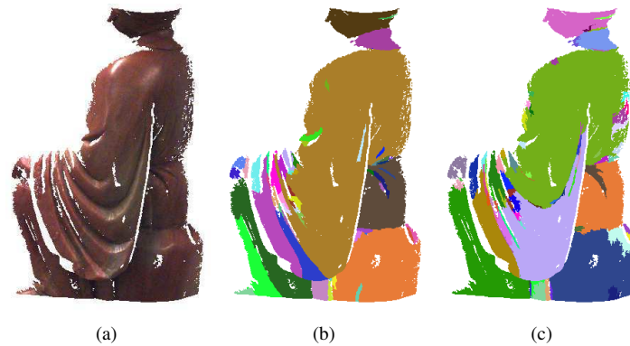
Fig. 3. Influence of the attribute space choice on the segmentation. Original range image (a). Segmented image in (b) angle between normal vector space, and (c) sphere fitting space.
