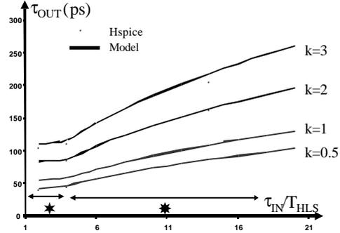
**Fig. 7.** Inverter output transition time ( $W_N=1\mu\text{m}$ ,  $W_P=2\mu\text{m}$ ,  $L=0.18\mu\text{m}$ ) loaded by 5 to 20  $C_{IN}$ .
