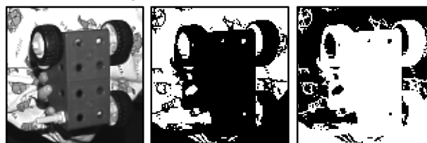
a. Greyscale reference image b. Positive reference image R[x, y] c. Negative reference image \bar{R}[x, y]
