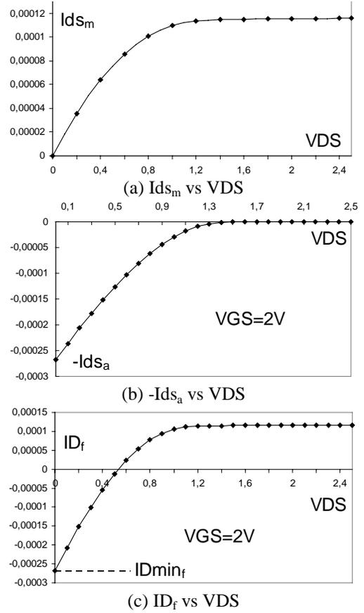
Fig.12: I-V curves in the non-linear non-split model
