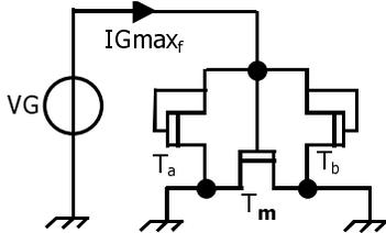
Fig.15: Equivalent circuit for the model at  $VDS=0$
