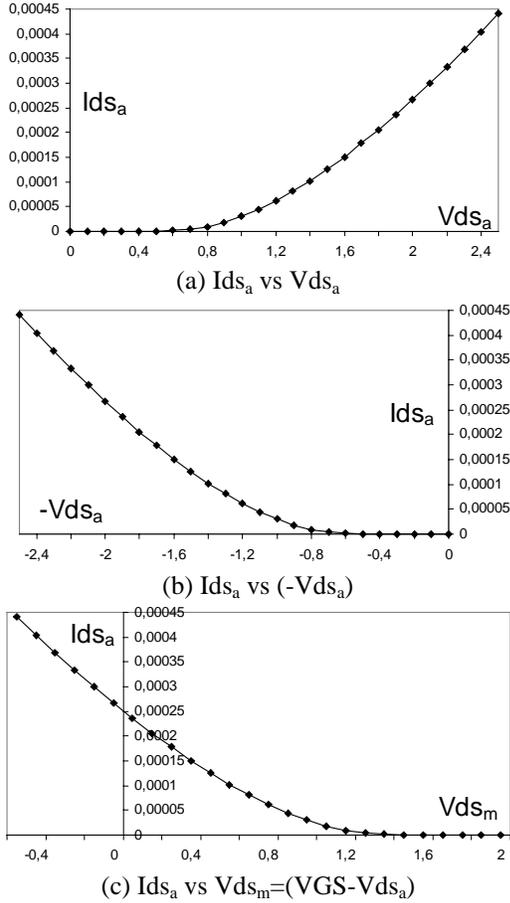
Fig.11: I-V characteristics of the additional transistor  $T_a$
