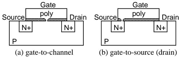
Fig.1: Pinhole in a MOS gate
