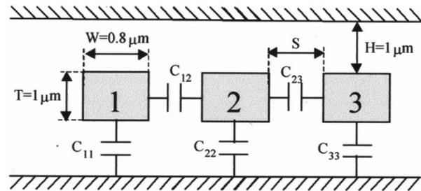
Fig. 6. Interconnection geometry.
