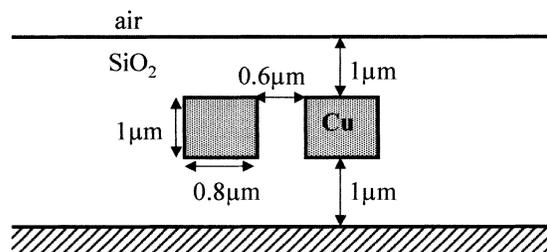
Fig. 1. Two coupled Cu lines.
