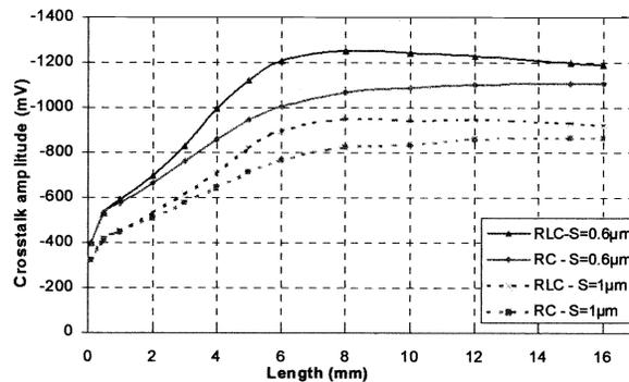
Fig. 9. Crosstalk amplitude variation versus interconnection length.
