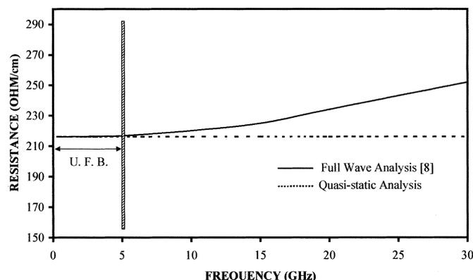
Fig. 2. Behavior of serie resistances of the two coupled lines.
