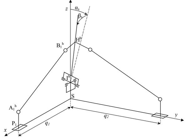
Figure 6 – Kinematic scheme of Twice upper part
