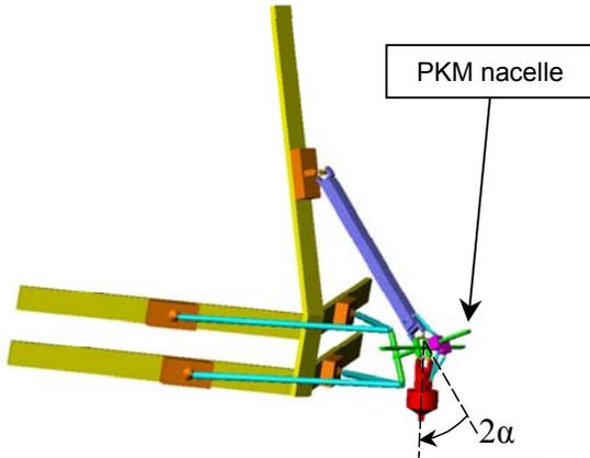
**Figure 2 – 5 dof parallel machine tool with Twice**
