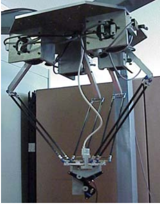
Figure 8. General view of H4 equipped with a redundant sensor, and a 3D measurement system
