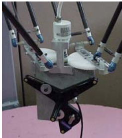
Figure 9. Closer view of the encoder and the 4-LED based measurement system
