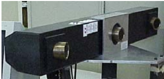
Figure 10. A view of the SAGEIS SM3D vision system with 3 linear CCD.
