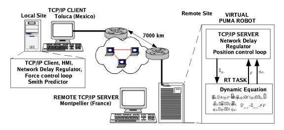
Figure 1 : Remote Position/Force Control of Virtual PUMA Robot
