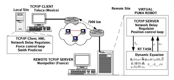
Figure 1: Remote Position/Force Control of Virtual PUMA Robot
